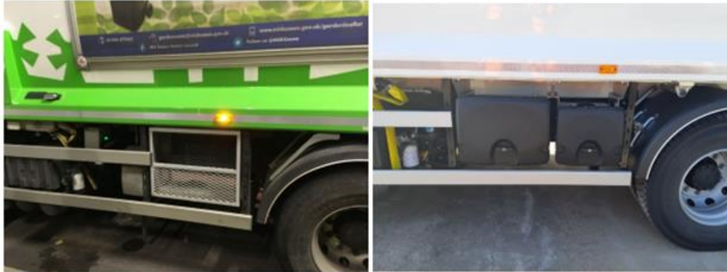
Figure 2: Examples of kerbside collection compartments on RCVs 205
